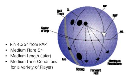
Balance holes can be used on all Fusion drilling techniques.
