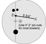
Note: Finger, thumb and X-holes must have at least a moderate bevel and the riser Pin (P) must be at least one inch from any drilled hole to comply with the Brunswick warranty
