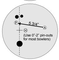
Note: Finger, thumb and X-holes must have at least a moderate bevel and the riser Pin nust be at least one inch from any drilled hole to comply with the Brunswick warranty
