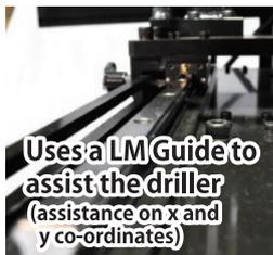
Uses a LM Guide to assist the driller (assistance on x and y co-ordinates)
