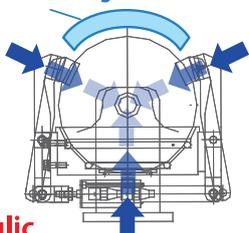
**World's first hydraulic clamping system for bowling balls.**
