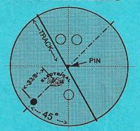
Place pin on center line of span or at 45° to vertical center line. Place **CG** on same line in thumb and negative quadrant. Place weight hole 3-3/8" below **CG** on same line.
