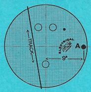
This layout produces maximum flair and maximum hook potential. Start with high top weight (3 oz.) Drill back to 3/4 positive side weight. Surface can be polished or dull.
