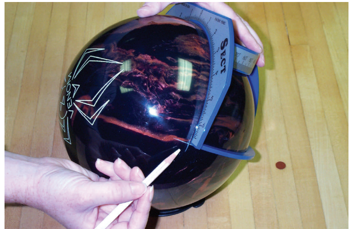
Step 2: Mark the opposite corner of the quarter scale on the surface of the ball at that 13 1/2" measurement.
