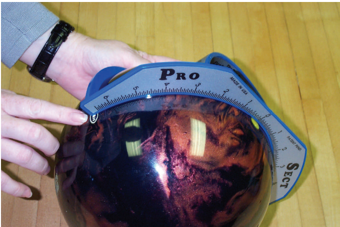
Step 1: Place one corner of the quarter scale on the marked mass-bias, and measure 13 1/2" through the pin of the ball.
